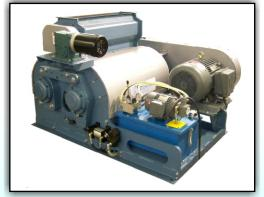
THE 36" TWIN ROLL HULLER & BASKET BEATER / SHAKER IS PRIMARY TO PRODUCE HULLS WITH A MINIMUM OIL CONTENT BY EFFICIENTLY BEATING THE HULLS TO REMOVE THE HIGH PROTEIN FINISHED MEATS.
