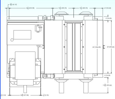
1] MAIN DRIVE MOTOR - 25HP 1450/1750RPM, 380/230/440V 50/60HZ
